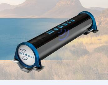
The Medusa Radiometrics MS-2000 scanner is a low-power, autonomous, and robust gamma-ray sensor developed with vehicle-borne mapping applications in mind. The housing is ultra-rugged, made of Kevlar-reinforced carbon fiber, and features a vibration-dampening mounting system. This system can be mounted on a variety of vehicles such as quad bikes, tractors, cars, and even larger drones.
