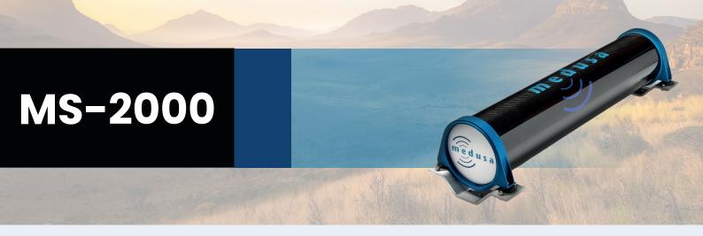
The Medusa Radiometrics MS-2000 scanner is a low-power, autonomous, and robust gamma-ray sensor developed with vehicle-borne mapping applications in mind. The housing is ultra-rugged, made of Kevlar-reinforced carbon fiber, and features a vibration-dampening mounting system. This system can be mounted on a variety of vehicles such as quad bikes, tractors, cars, and even larger drones.
